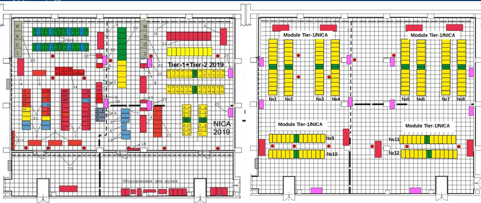
Schematic arrangement of the equipment in the computer hall at the 2-nd and 4-th floors
